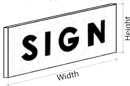
FIGURE 12-1: MEASUREMENT OF A SIGN FACE
